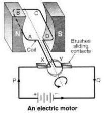
When the coil is in vertical position, the brushes X and Y would touch the center of the commutator and the current in the coil is stopped. Though current is stopped but the coil comes back in horizontal state due to momentum.
