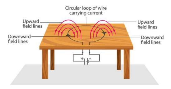
For the downward direction of the current, the direction of the magnetic field will be as if emerging from the table outside the loop and merging with the table inside the loop. Similarly, for current flowing in an upward direction, the direction of the magnetic field will be as if they are emerging from the table outside the loop and merging with the table inside the loop.
