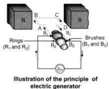
**Working:** When the armature coil ABCD rotates in a magnetic field produced by the permanent magnets, it cuts through the magnetic lines of force.
